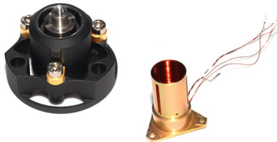
Figure 6 – Voice coil assembly (magnet on the left, coil on the right)
